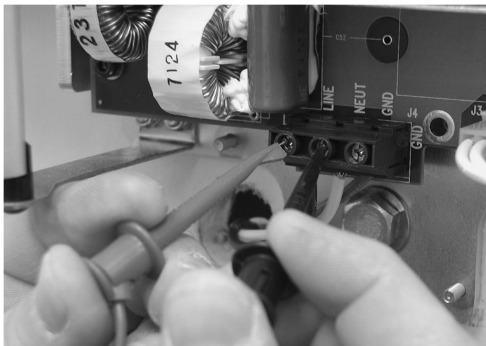
Figure 31 Verifying Input Voltage at the Line Input
