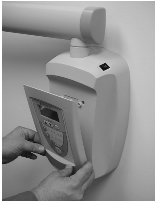
Figure 37 Snapping in the Operator Panel
