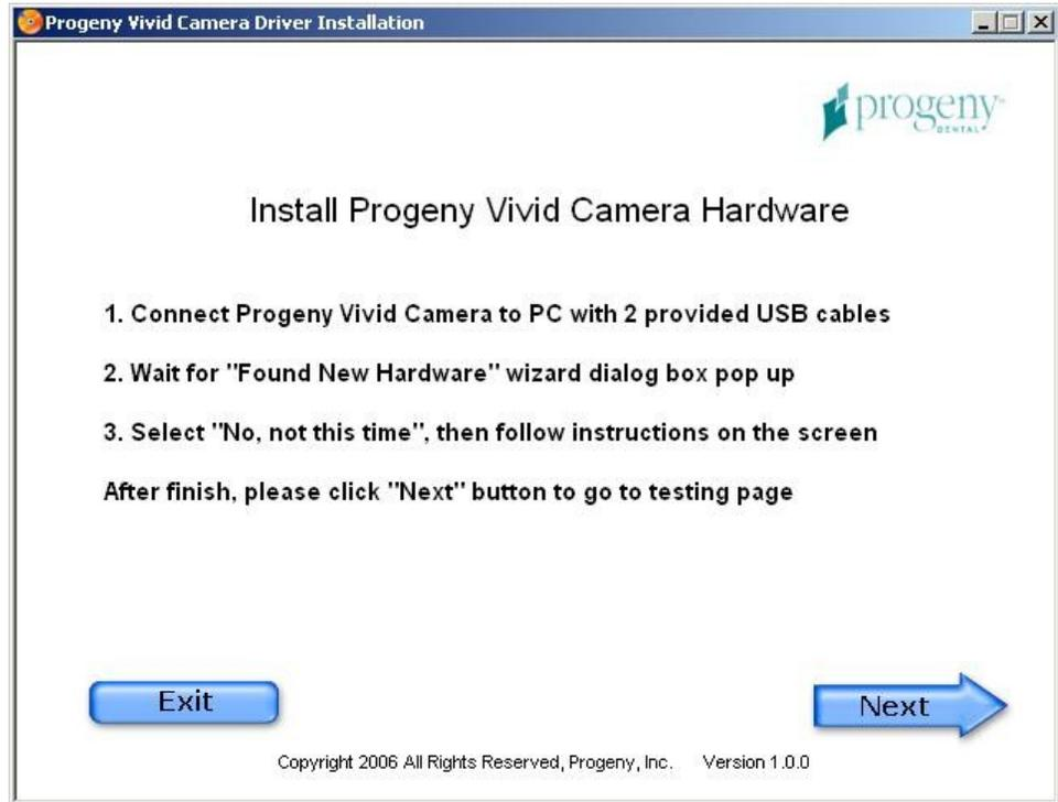
4. Connect the two USB cables to the USB ports on the USB hub and to the USB ports on the USB video converter. Several messages will appear indicating that new hardware has been detected, and the Found New Hardware Wizard will appear.
