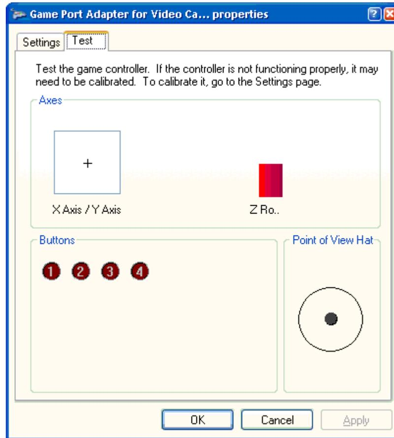
3. While this window is in the foreground, press and release the capture button on the Vivid Camera Handpiece. The "1" button should flash
