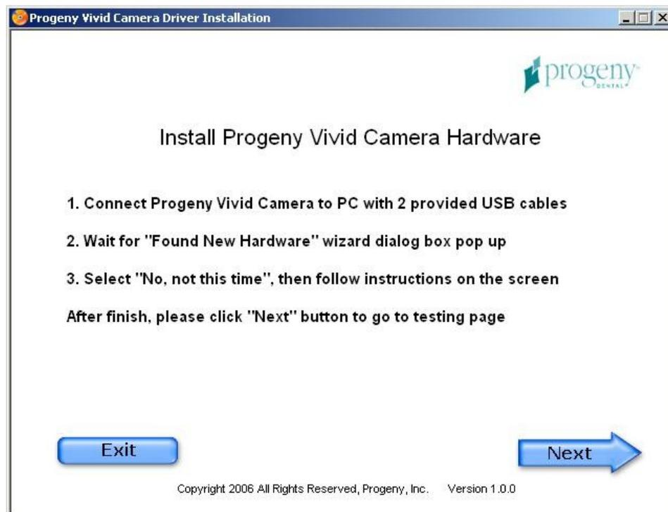
4. Following the instructions on the screen, connect the two USB cables to the USB ports on the computer and to the USB ports on the USB video converter. Several messages will appear indicating that new hardware has been detected, and the Found New Hardware Wizard will appear.
