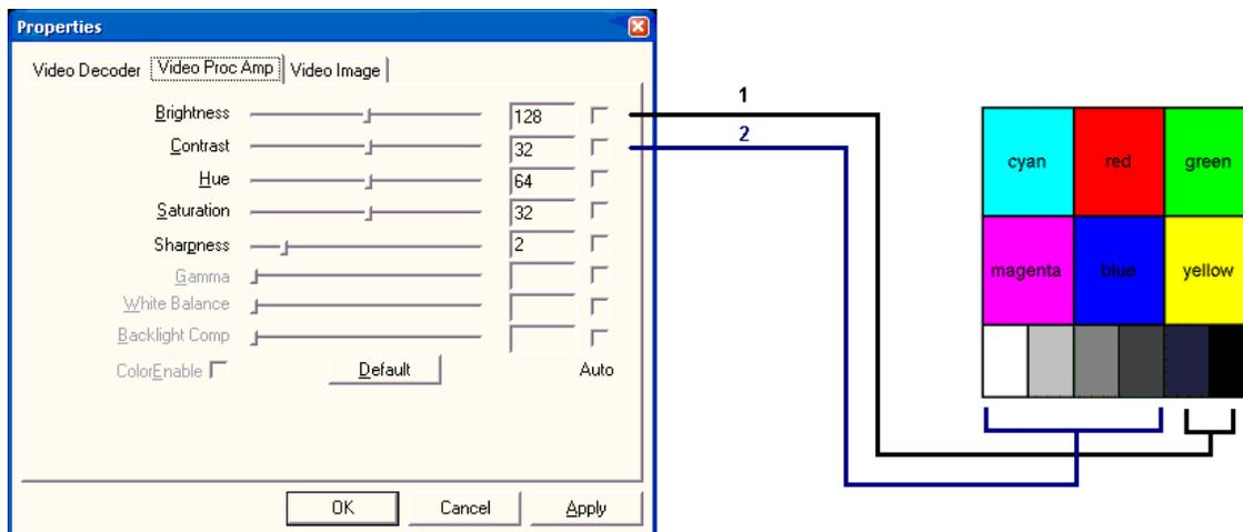
4. Place the Blue-only Switch in the **ON** position. The entire computer monitor display will appear in shades of blue.
