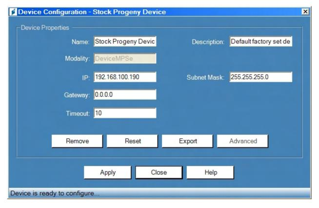
The Device Configuration screen allows you to configure an image acquisition module. Changes made on this screen are stored in the module's non-volatile memory and will affect all clients (users) of this module.
