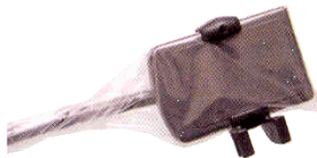
Figure 4: Using protective sensor sheath
