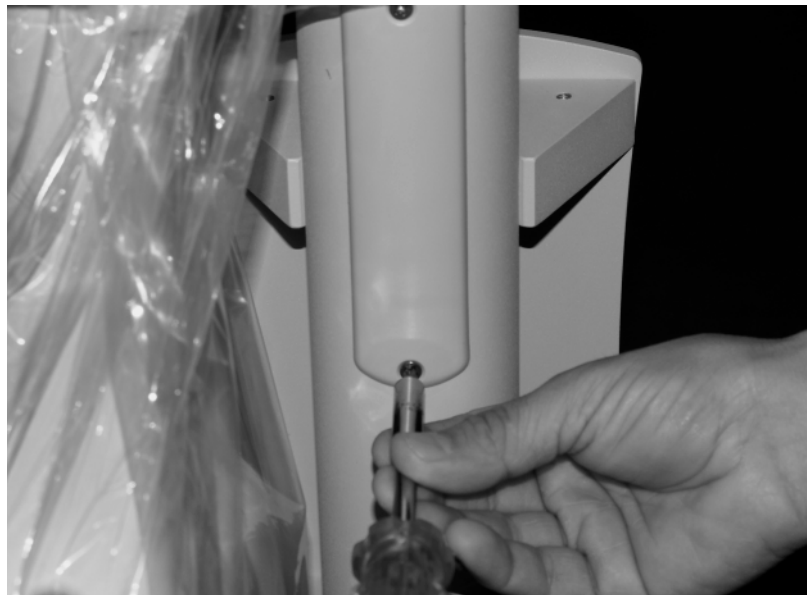
Figure 29: Re-installing the Access Plate to Vertical Column
