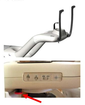
**15.** You can now turn on the Vantage by pressing the on/off switch located at the back of the stationary column. Make sure that all shipping brackets have been removed.
