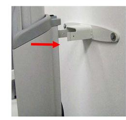
CAUTION! The snap partially secures the Vantage panoramic device. The following clamps and floor mount steps must be completed to hold the device in place.
