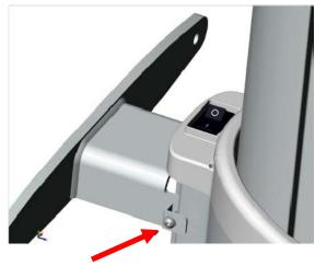
**7.** Hold a level vertically against the column and move the Vantage panoramic device on the floor until it is leveled. Do a final level test before completely tightening the clamp screws.
