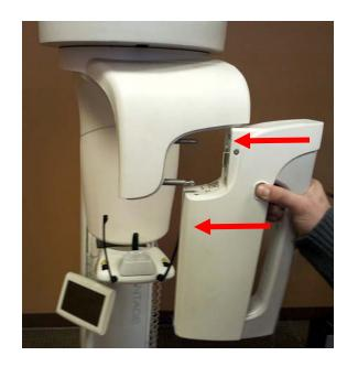
**14.** Install the chin rest, bite guide and temple wands. Before energizing the system, make sure the emergency stop switch has not been pressed. If so, rotate the switch until it is released.
