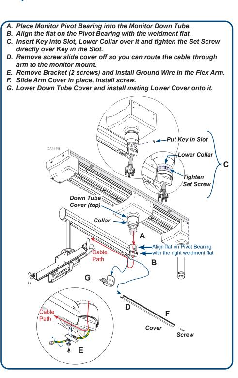
**Step 5** Attach the Light Flex Arm to the Down Tube.
