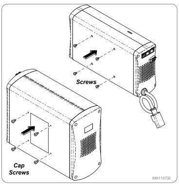
Step 4: Position battery using cap screws to hang battery to power mount assembly.
