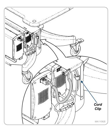
Step 8: Mount RUI Display onto pole assembly with screws (2).
