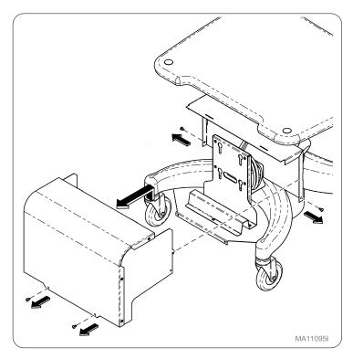
Slide charger into rear of power mount assembly using screws to hang charger to assembly and tighten screws (4).
