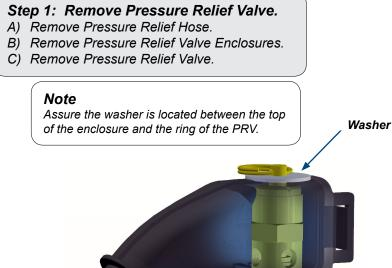
**Note** The Pressure Relief Valve has a seal on the threads to prevent leakage.
