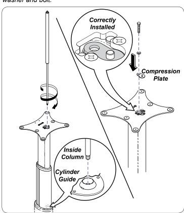
**Step 6:**Remove bolt, washer and compression plate. Rotate current gas cylinder to remove from column.
