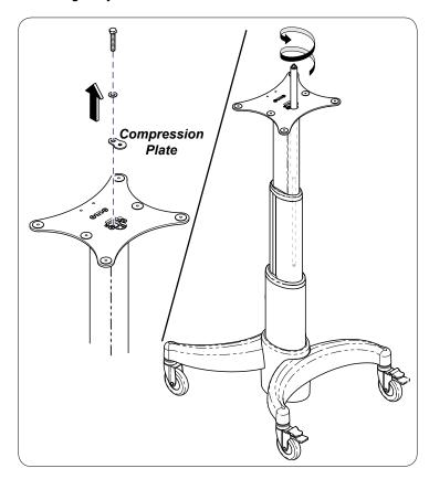
**Step 8:**Secure and worksurface to mounting plate with screws (6).
