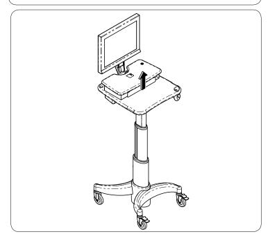
**Step 4:**If necessary remove any accessories blocking access to mounting plate.
