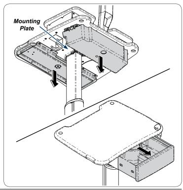
**Step 5:**Remove screws (6) and worksurface from mounting plate.
