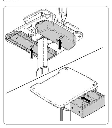
**Step 16:**Before testing Workstation be sure all components are mounted. Press hand actuator paddle to adjust.
