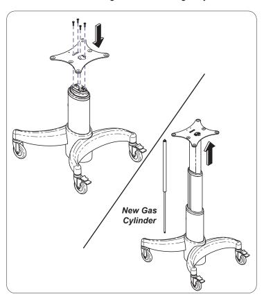
Step 12: Secure and worksurface to mounting plate with screws (6).
