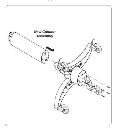
**Step 11:**Rotate replacement gas cylinder into position in column and tighten. Secure by installing compression plate washer and bolt.
