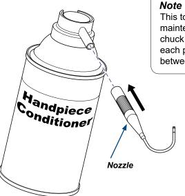
This tool is used in a portion of the maintenance process for appropriate handpieces. For complete maintenance procedures, refer to the user guide. For best results, clean and lubricate push button and chuck during each complete handpiece cleaning. Complete handpiece cleaning is recommended after each patient to mitigate cross contamination between patients. This procedure may also be performed between handpiece cleanings if the handpiece appears to be under performing.
