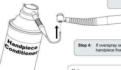
If overspray on the towel appears discolored repeat spray for an additional two seconds. Remove the handpiece from the nozzle tip and wipe excess conditioner from handpiece with clean dry towel.
