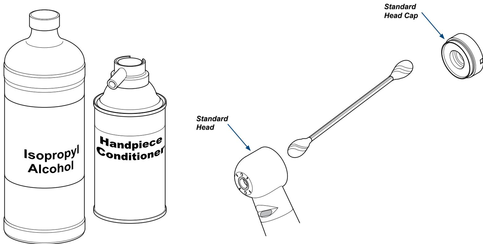
**Step 7:** Apply handpiece conditioner to entire area of head and interior of the new head cap.
