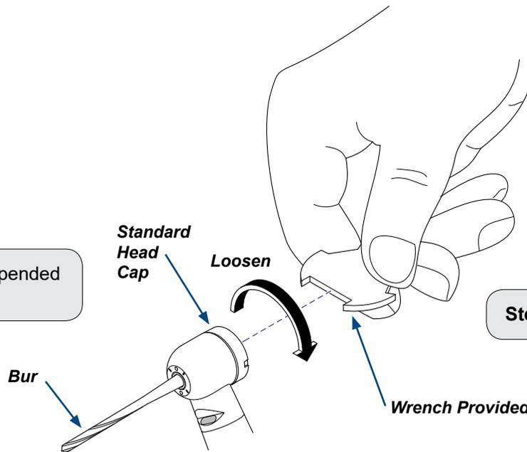
**Step 3:** Loosen head cap with wrench provided.
