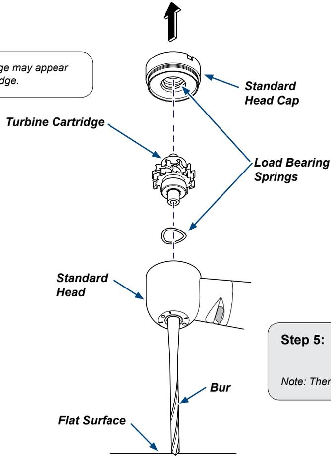
*Note: If bur doesn't rotate or spin the turbine cartridge is installed improperly or there is another component causing malfunction, contact Midmark Technical Service or authorized dealer.*
