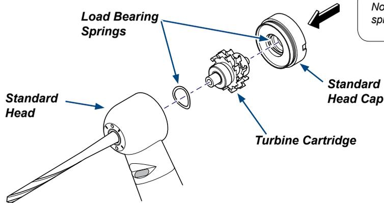
Note: Verify there is a load bearing spring and o-ring in the new head cap.
