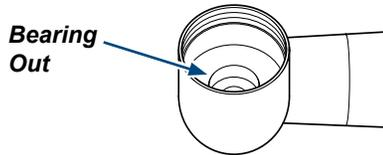
**Step 5:** Discard worn turbine cartridge, head cap, and load bearing spring from inside head.
