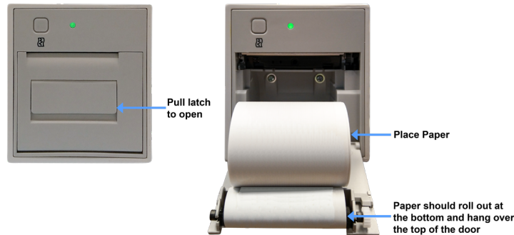
Printer and paper installation guide (Fig. 5.6.6-1)
