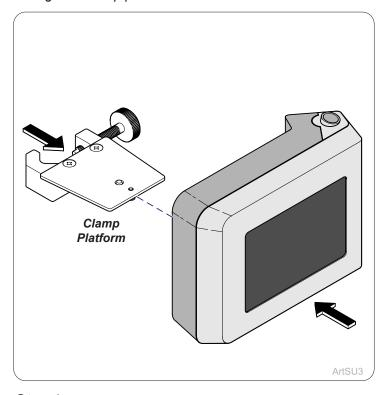
**Step 4:**Place clamp onto cuff holder pole and tighten thumb screw.
