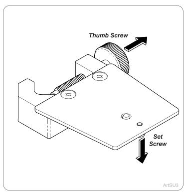
**Step 3:**Ensure button snaps into bottom of device and hand tighten set screw may need to tighten with allen wrench.
