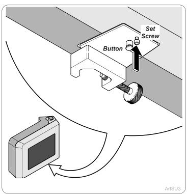
**Step 2:**Assemble Clamp and Digital Vitals Signs Device by sliding onto clamp platform.
