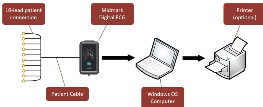
Block Diagram of the Midmark Digital ECG system
