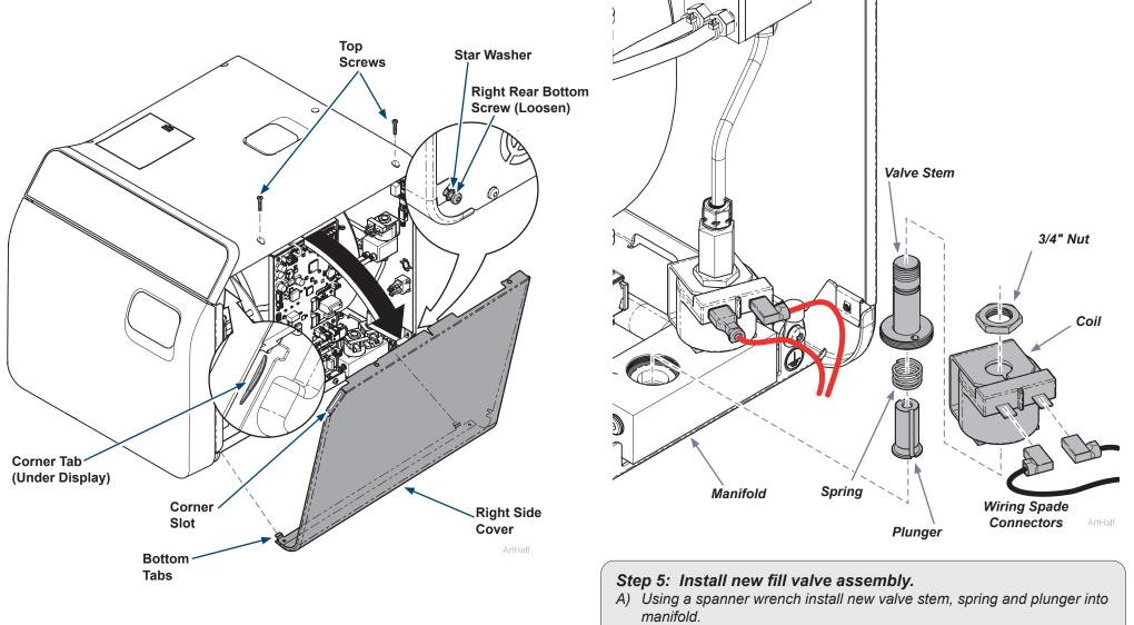
*B)* Install coil onto valve stem and secure with 3/4" nut. Attach wiring spade connectors to coil.
