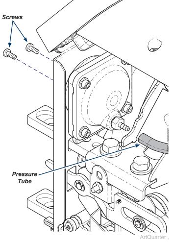
Step 5: Remove Interlock assembly.
