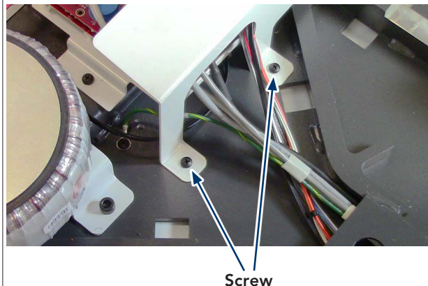
Step 12: Remove two screws and fluid ingress bracket.
