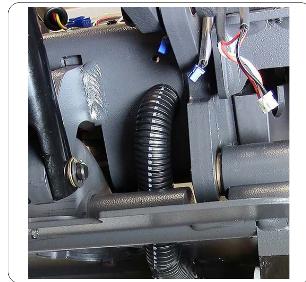
Step 19: Ensure wire shielding is in place when routing harness into seat weldment.
