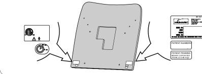
The labels on the standard back support board are <u>es</u>-<u>sential</u> for model identification and regulatory compliance.
