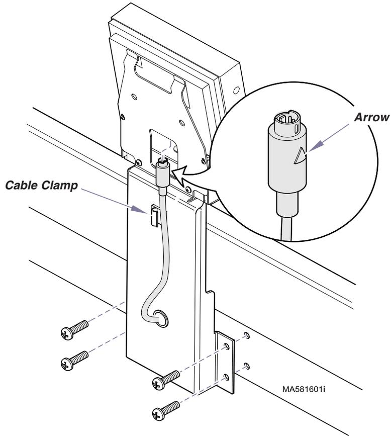
**Step 3: Provide power to digital scale.**
