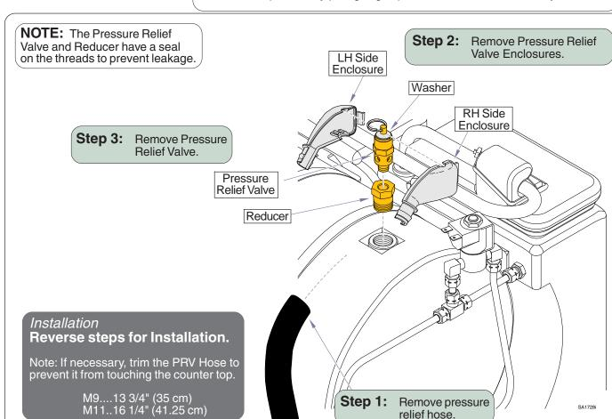
NOTE: Assure the washer is located between the top of the enclosure and the ring of the PRV.
