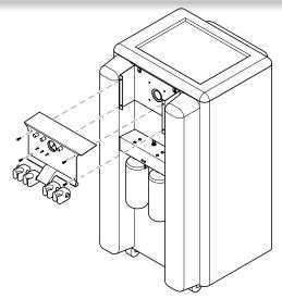
Units with Serial Numbers beginning with VxxxxxStep 6: Remove four screws from top panel.
