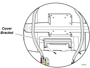
**Step 3:** Mount the new cover bracket to the mounting plate using the same two screws.
