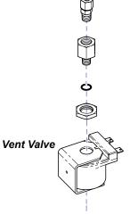
Step 4: Disassemble valve and remove any debris.
