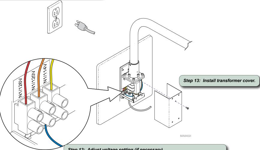
Step 12: Adjust voltage setting (if necessary).
