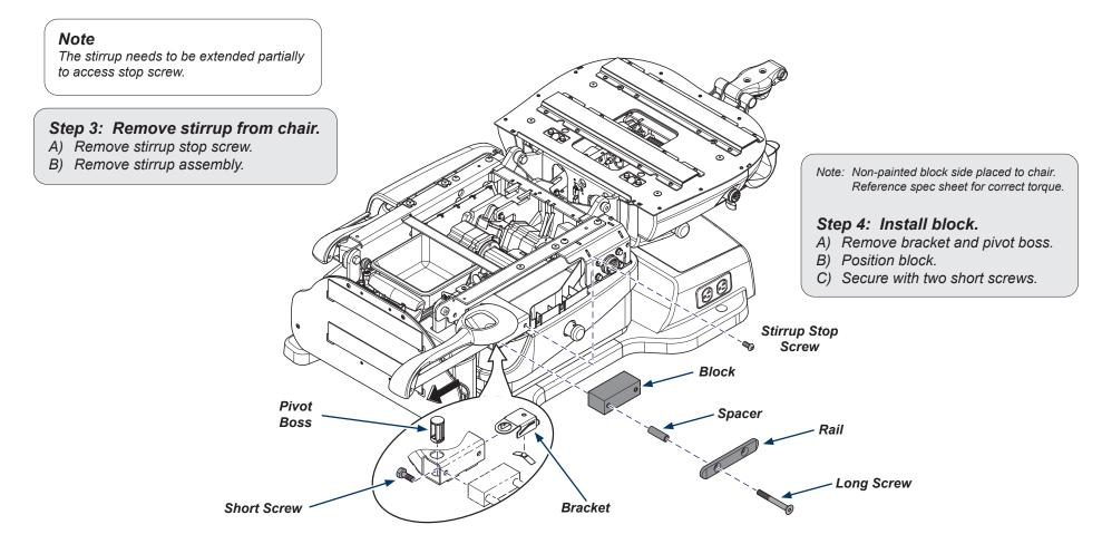
Note: Reference spec sheet for correct torque. Place rail with large hole on outside so long screws are flush with rail.
