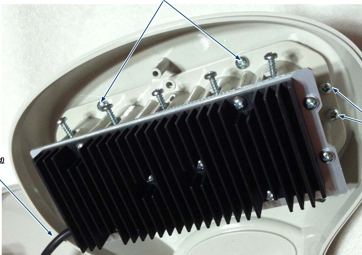
Screw Locations (One of Two Long Sides Shown)
