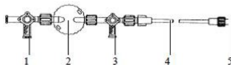
Fig. 11-1 IBP Transducer Connection Diagram
