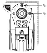
Position pins as shown to limit rotation to the right
