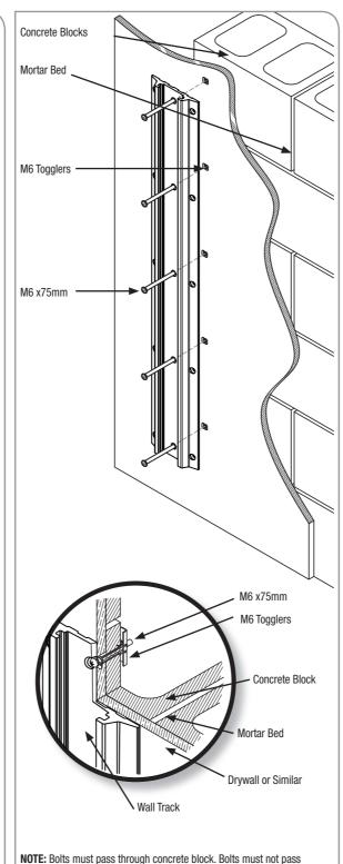
through mortar bed between blocks nor through the web within the blocks.
