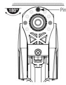
Position pin at 12:00 to prevent the arm from coming in direct contact with the wall on either side
