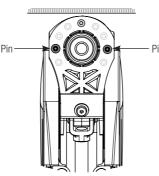
Position pins at 3:00 & 9:00 for a full rotation lock out
