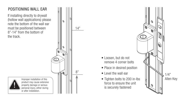
We recommend having the wall ear installed at the following heights which comfortably accommodates the majority of users in seated or standing positions.
