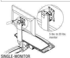
Mount the monitor directly to the VESA plate on the Float Tower with the the four screws provided. (Choose either short or long screws for your application.) Use a #2 Phillips screwdriver to secure.
