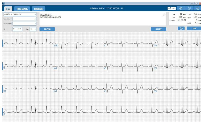
**NOTE:** Interpretation algorithm: Midmark ECG Analysis Program. The duration measurement of Q-wave, R-wave or S-wave does not include the iso-electric segments within the global QRS complex.
