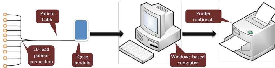
Figure 1 Block Diagram for the IQecg® system
