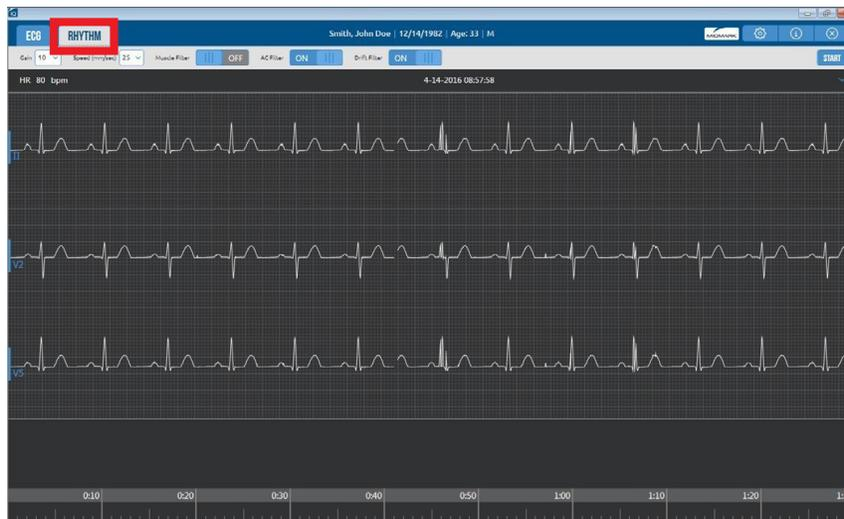
The gain, speed and filter settings are displayed above the moving tracings. Click the appropriate drop-down item, or toggle to modify its setting. Use the drop-down list on the left-side of each tracing to change the rhythm leads. Changes to these settings made from this screen are temporary and only apply for as long as the test is active. You can make changes and set them as the default settings for all new ECG tests by clicking **Settings**.
